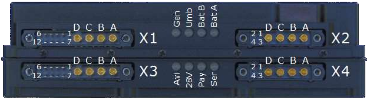
Figure 1 – Locations of connectors and visual indicators on the front panel
