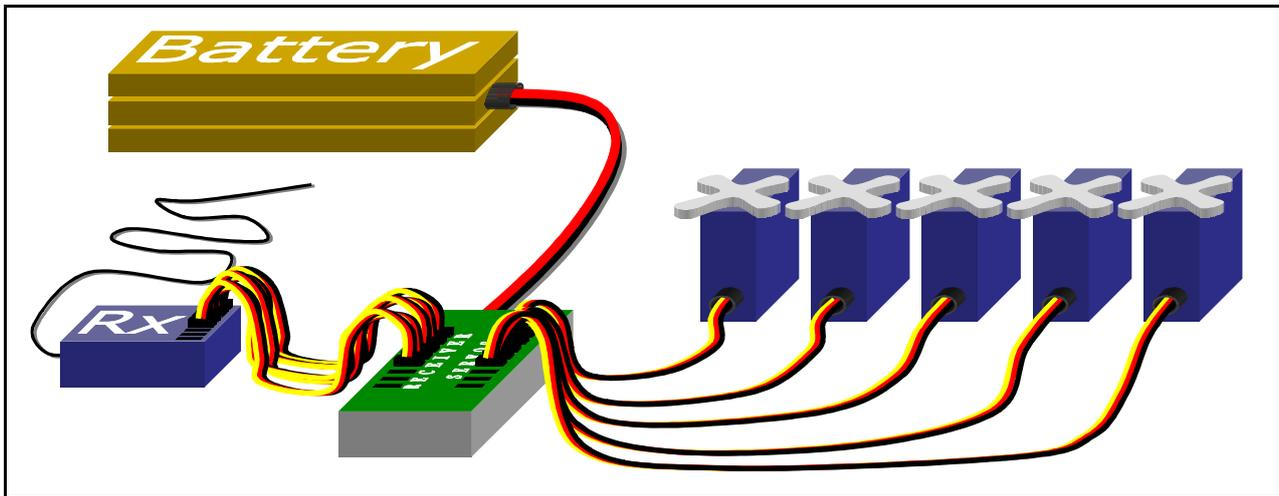
**Fig. 2: A typical 5-channel setup for fuel powered vehicles**
