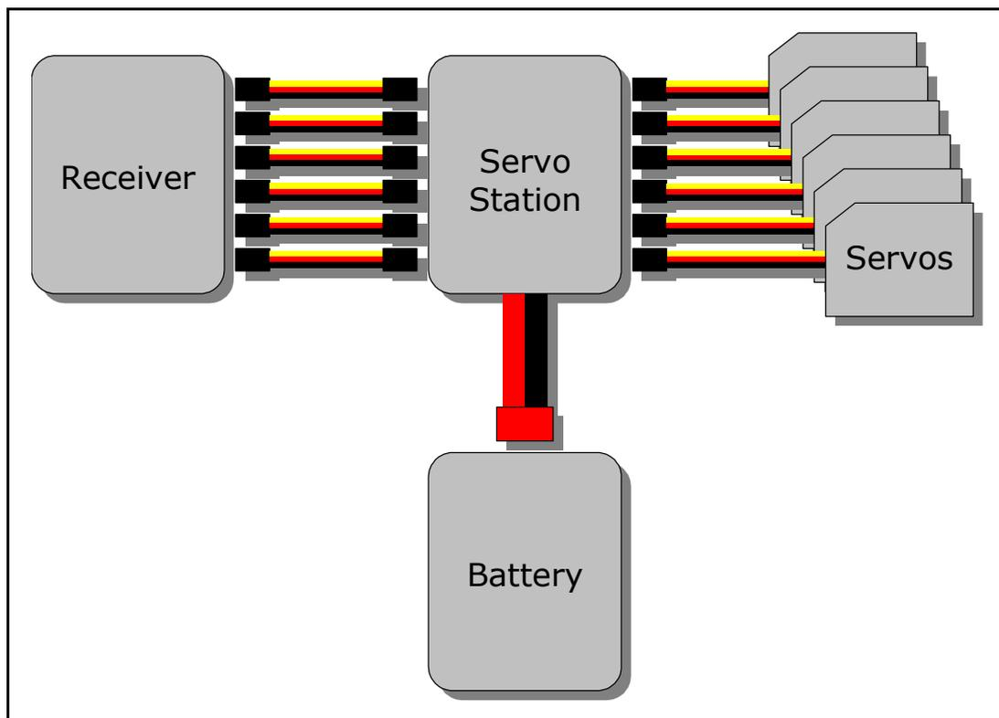
**Fig. 1: ServoStation connections**
