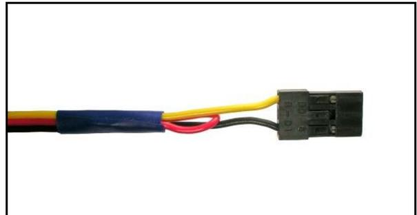
**Step 4:** Secure the wire and pin with some insulating tape or heatshrink tubing.
