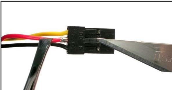
**Step 2:** Lift up the plastic tongue and pull out the middle wire with its pin. Tweezers and a third hand are useful.
