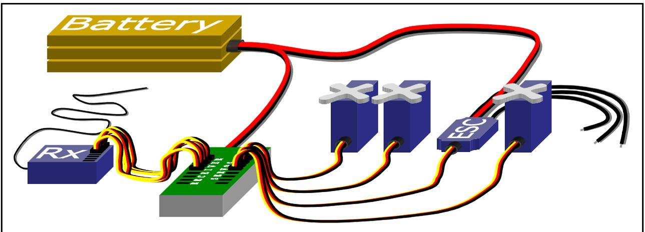
**Fig. 3:** A typical 4-channel setup for electric powered vehicles
