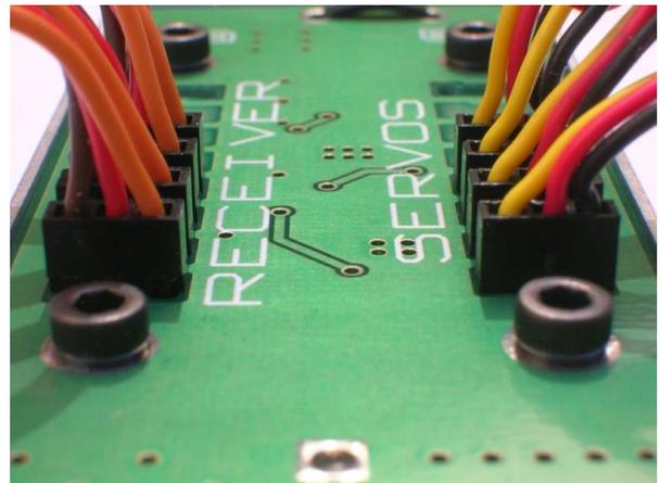
**Connect your receiver to the ServoStation using one receiver cable per channel. The 8 channels provided by the ServoStation are all identical and may be arranged in any order.**
