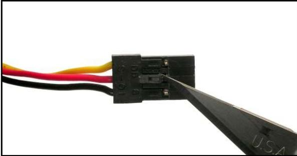
**Step 1:** Insert a scalpel blade behind the middle plastic tongue of the ESC's receiver connector.
